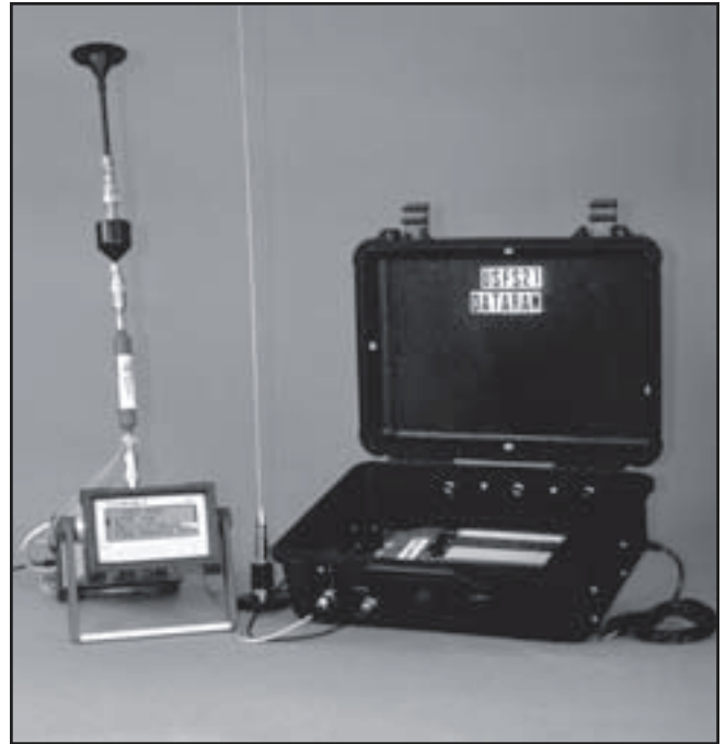
Figure 6—DataRAM4 connected to the telemetry unit.
