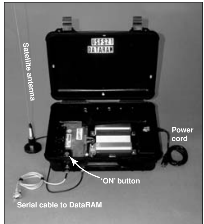
Figure 5—Remote telemetry unit used with the DataRAM4.
