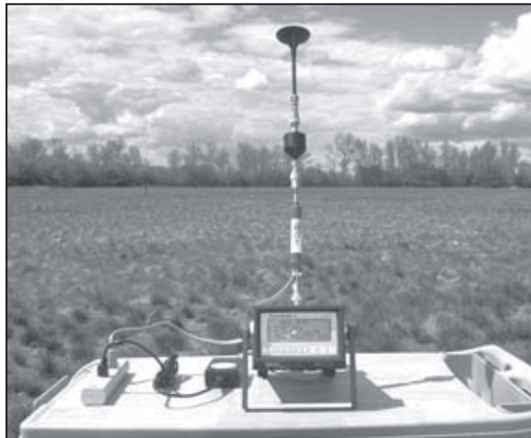
The DataRAM is sited in an open field for collecting smoke data.
